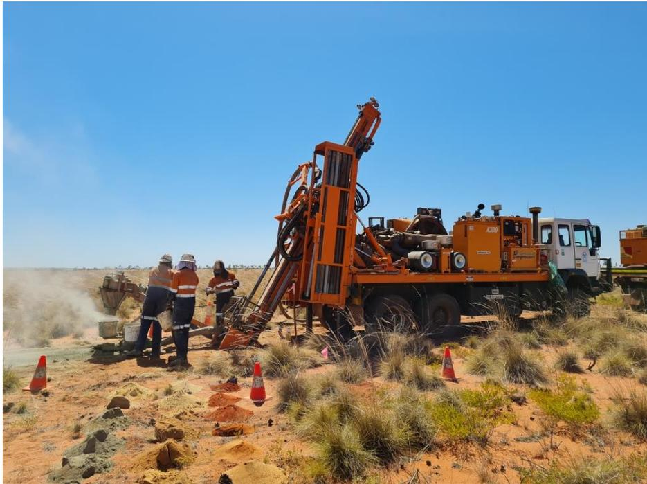
**Figure 1: Photo of first Aircore drill hole at the Palisade prospect in the Mallina Basin, Pilbara, WA.**
