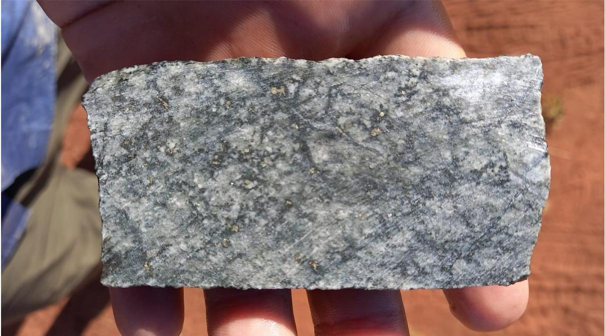
**Figure 1. Bastion Prospect drill core photo from PLDD0005, 174.4m depth, 1.1 g/t gold hosted by disseminated sulphides in an intrusion.**
