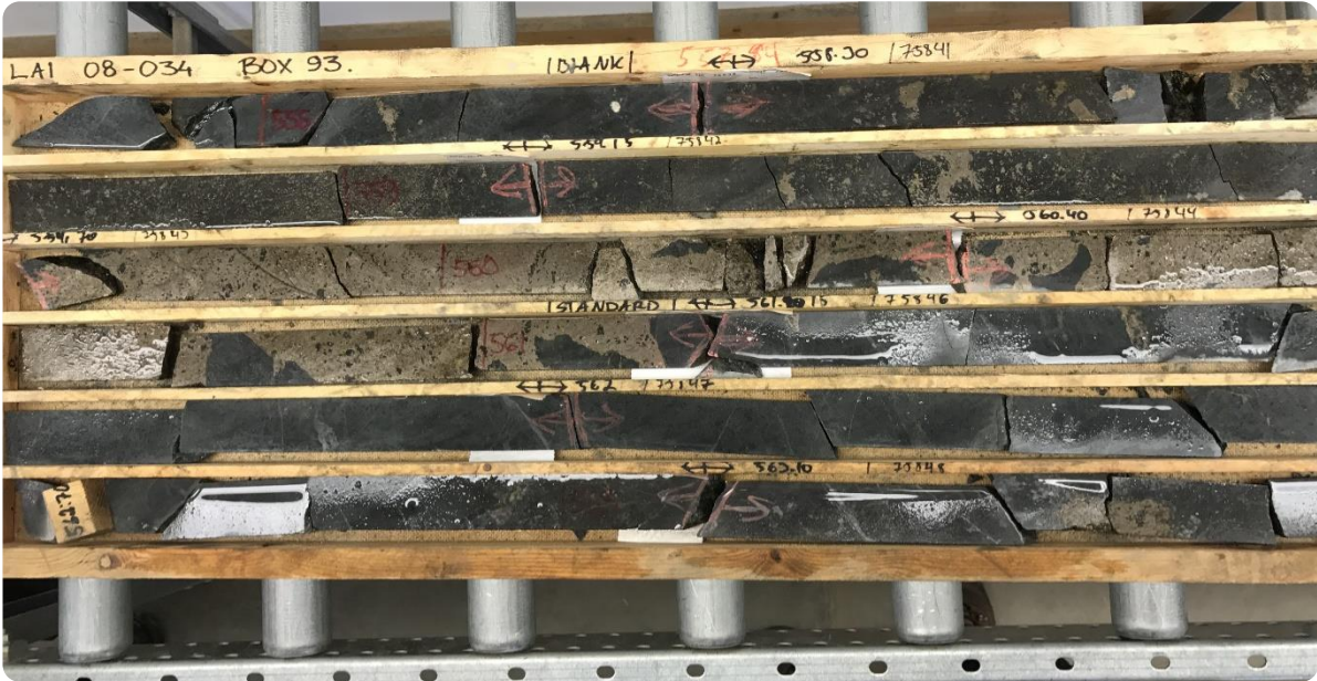
LAI08-034 (from 559m) 2m @ 2.14% Ni, 0.038% Cu and 0.09% Co - open to north
